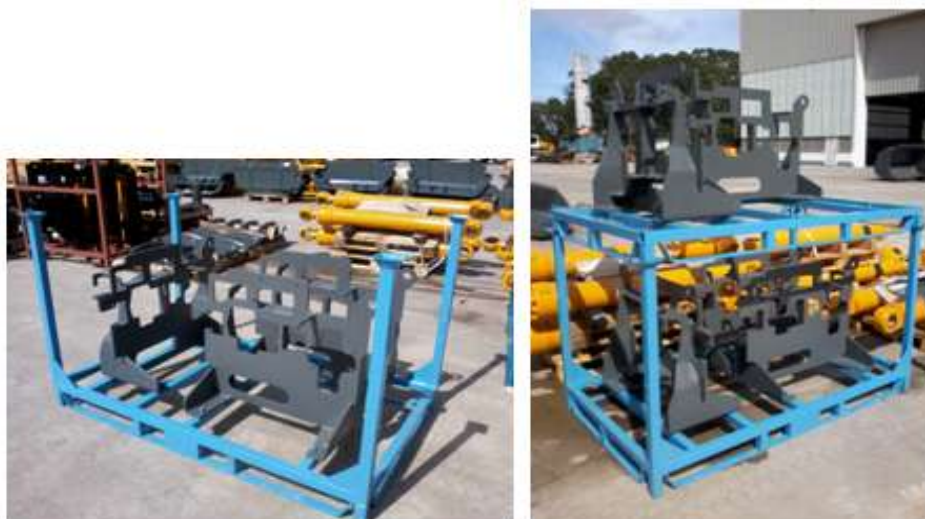
(a) (b) Figure 2 (a) and (b) - New rack for supporting the valve block Source: Authors
