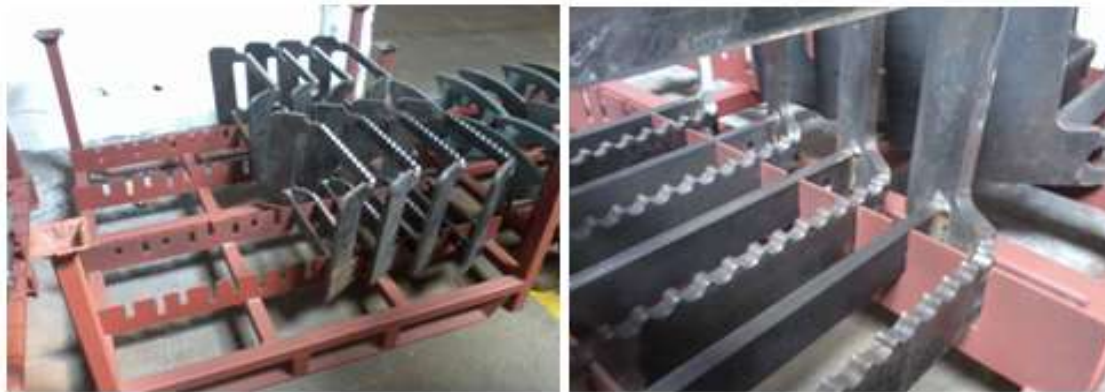
(a) (b) Figure 4 (a) and (b) - metallic rack for stirrups in experimentation
